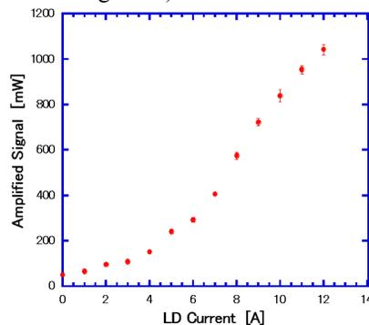
Figure 5: Fiber Amplification Test Result
