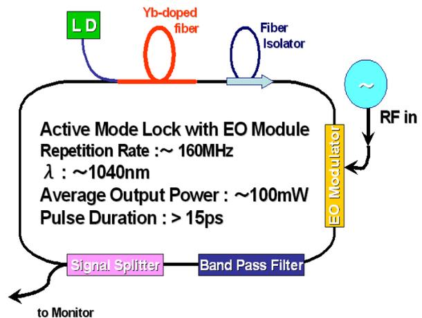
Figure 1: Layout of Oscillator
