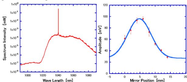
Figure 3: Spectrum and Pulse Duration of the Oscillator
