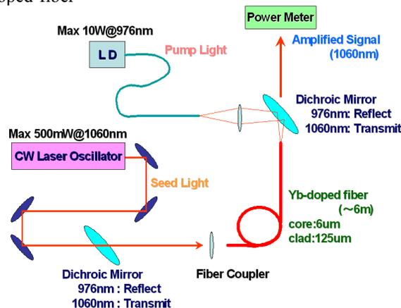
Figure 4: Fiber Amplification Test Setup
