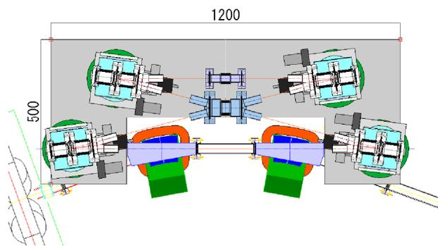
Figure 6: Top View of External Optical Cavity
