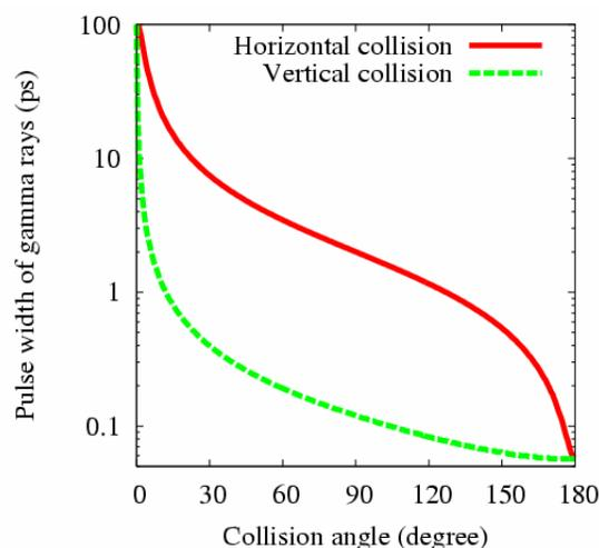
Figure 1: Dependence of the pulse width of the gamma rays on the collision angle. Solid line shows the horizontal collision which the laser is injected from the direction in the orbital plane. Dashed line shows the vertical collision which the laser is injected from the direction to the orbital plane.
