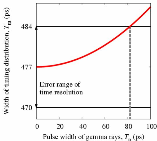
Figure 2: Relationship between the width of the timing distribution measured by the MPPC module and the pulse width of gamma rays for negligible time jitter (thick solid curve). Thin solid line shows the error range of the time resolution. Dashed line shows the shortest pulse width that the MPPC can evaluate.
