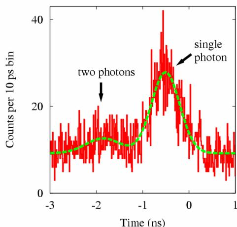
Figure 4: Experimentally obtained timing distribution between gamma rays and trigger signal. Dashed curve shows a result of Gaussian fitting. The width of the single-photon distribution is  $720 \pm 30$  ps (FWHM).
