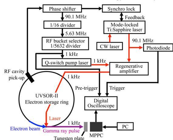
Figure 3: Schematic representation of the experiment.
