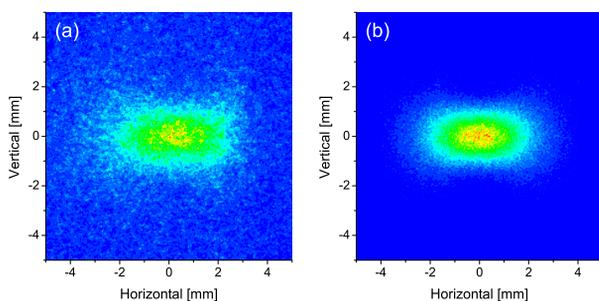
Figure 2: (a) Measured and (b) simulated spatial distributions of LCS gamma-rays.
