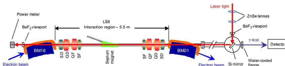
Figure 1: Experimental setup for LCS gamma-ray generation at the SAGA-LS storage ring.
