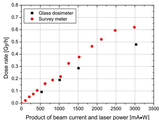
Figure 3: Effective dose rate of LCS gamma-rays in the irradiated area. The dose rates were measured using a glass dosimeter and a survey meter.
