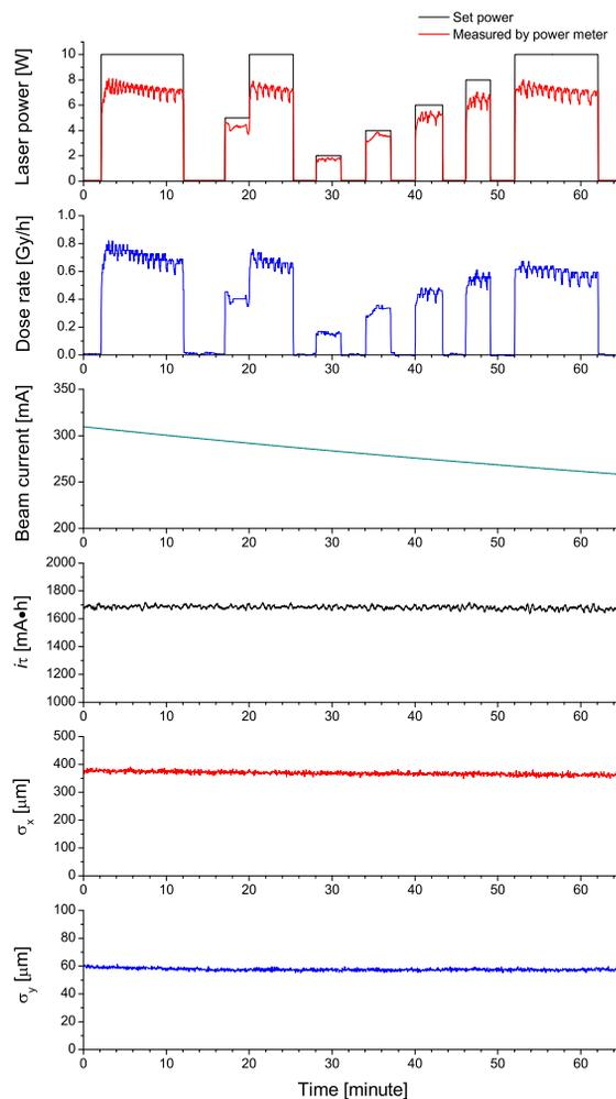
Figure 4: Laser power, dose rate, and beam parameters (i.e., beam current, product of the beam current and lifetime, and transverse beam sizes) recorded during LCS gamma-ray generation.
