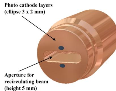
Figure 2: Copper cathode plug.
