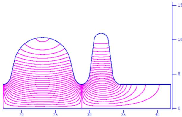
Figure 5: RF field of reduced beta end cell ( $\pi$ -mode).
