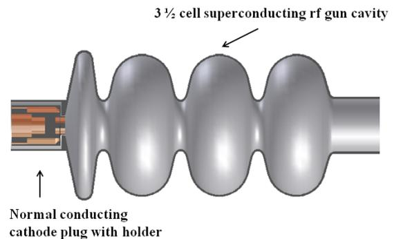
Figure 1: Cross section of the SRF gun cavity.
