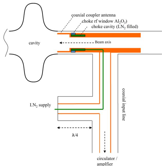
Figure 6: Layout of LN<sub>2</sub> choke HOM damper.
