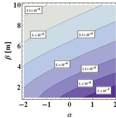
Figure 5: Analytical calculation results of emittance as function of twiss parameter at the entrance of merger
