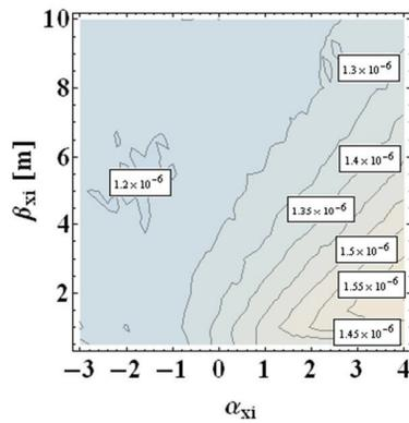
Figure 6: Transverse emittance at the exit of the merger as function of the initial  $\alpha_{xi}$  and  $\beta_{xi}$ .
