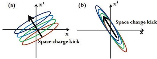
Figure 3: Growth of projected emittance due to the SC effect in merger section. (a) Maximum case of projected emittance growth (b) Minimum case of projected emittance growth
