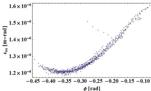
Figure 7: Transverse emittance at the exit of merger section as a function the orientation of the phase ellipse.
