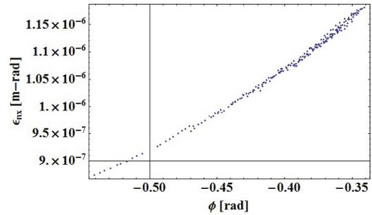
Figure 8: The change of transverse emittance at the exit of merger section as function the orientation of the phase ellipse due to the change of vertical CS parameters.
