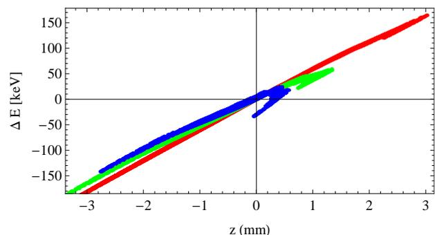
Figure 3: ALICE simulated injector longitudinal phase space as a function of BC1 phases. BC1= $-20^\circ$  (red),  $-10^\circ$  (green),  $-5^\circ$  (blue).
