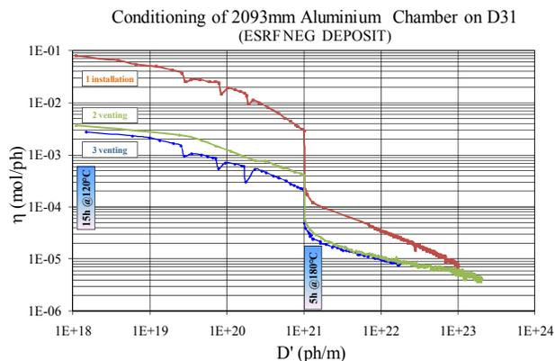
Figure 5: Repeated activation test. After each test the chamber was vented. The initial yield was progressively lower. The step behaviour is due to NEG activation.
