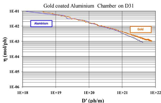
Figure 3: Photodesorption yield of a bare aluminium chamber and the same chamber with a gold coating
