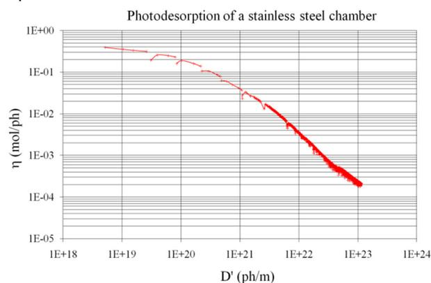
Figure 4: Wall pumping effect on a stainless steel chamber. The breaks show the effect of improved pumping after beam is restarted.
