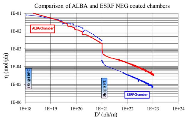
Figure 2: Activation of an ALBA chamber coated by SAES Getters and an ESRF chamber coated at ESRF
