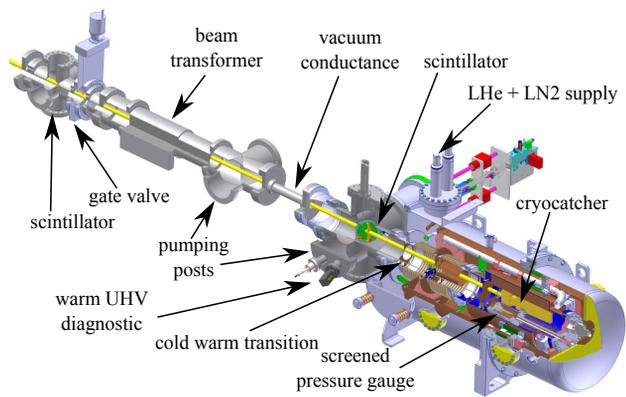
Figure 3: 3D-sctech of the prototype cryocatcher test setup.
