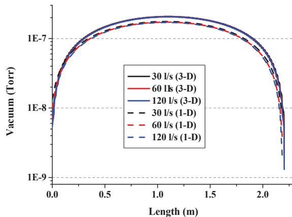
Figure 4: Vacuum pressures with pumping speeds.
