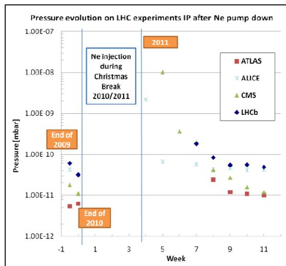
Figure 2: Pressure evolution after the Shutdown of 2010.
