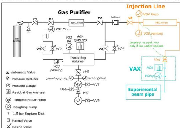
Figure 1: Schematic of the Gas Injection System for ATLAS, CMS and ALICE.
