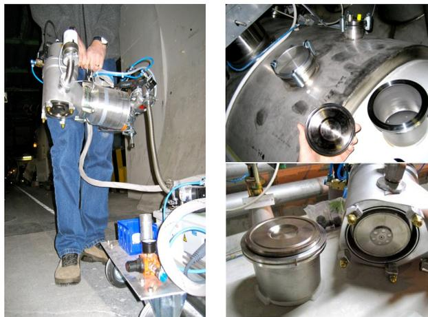
Figure 3: Additional turbo pump mounting on magnetically coupled flanges.
