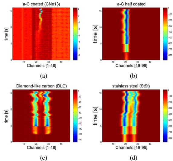
Figure 3: Comparison of the electron signal measured with ECM at a magnetic field of 0.12 T with LHC type beam of 3 batches at 25 ns bunch spacing in the SPS on: (a): a-C coated liner (CNe13) kept in the SPS since August, 2008 (CNe13). (b): Half coated with a-C on bare stainless steel (CNe70 half coated). (c): Diamond-like carbon coating (DLC, KEK). (d): Stainless Steel (StSt).
