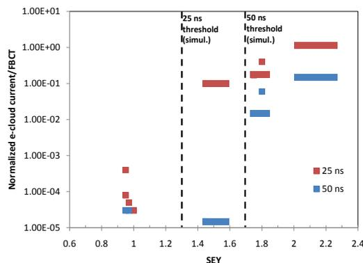
Figure 6: Normalized ECM signals as a function of SEY.
