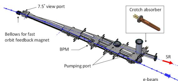
Figure 1: Layout of a B1 bending vacuum chamber
