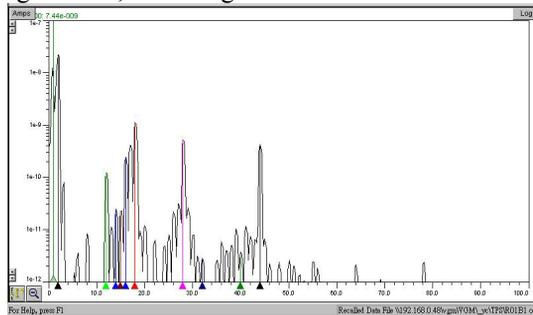
Figure 5: Mass spectrum from the RGA after a baking test. Major residual gases are  $H_2$ , C,  $H_2O$ , CO and  $CO_2$ .
