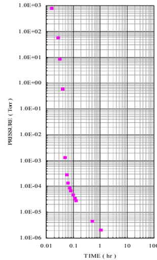
Figure 2: Pressure of chamber R01B2 after welding; the slope of the pumping curve is proportional to  $t^{-1}$ .
