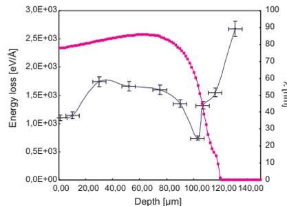
Figure 3: Depth evolution of the phonon mean free path ( $\lambda$ ) along the ion trajectory, for carbon fibers in AC150 carbon-carbon composite sample, exposed to  $1 \cdot 10^{13}$   $^{238}\text{U}$  ions/cm<sup>2</sup>, 11.1 MeV/u. The minimum value for  $\lambda$  corresponds to the elastic collision domain.
