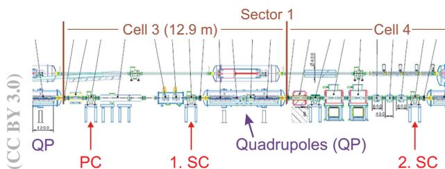
Figure 5: Position of proton collimation system sector 1 of the SIS100 lattice. PC denotes the primary collimator, 1.SC and 2.SC denote the 1st and 2nd secondary collimator, respectively.
