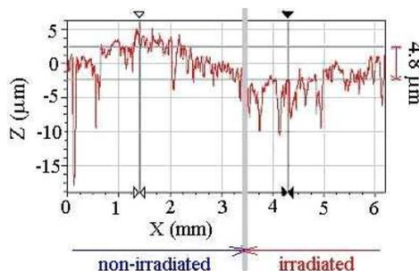
Figure 1: Profilometer scan across the pristine-irradiated border of a AC150 carbon-carbon composite sample, exposed to  $1 \cdot 10^{13}$   $^{238}\text{U}$  ions/cm<sup>2</sup>, 11.1 MeV/u, showing out-of-plane contraction of irradiated part.
