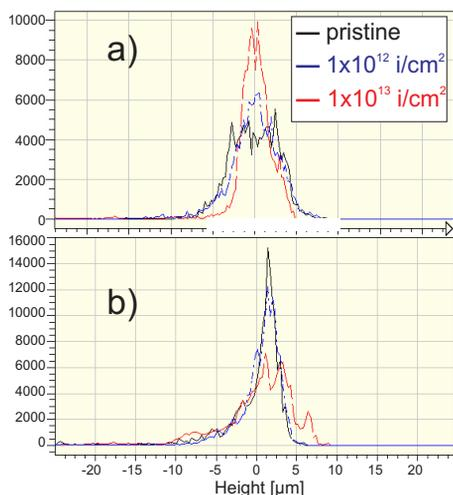
Figure 2: Histograms of roughness for profilometer mappings on the irradiated surface of two different AC 150 C-C composite samples cut along perpendicular orientations of the fibers and exposed to  $1 \cdot 10^{13}$   $^{238}\text{U}$  ions/cm<sup>2</sup>, 11.1 MeV/u, different fluences: a) in-plane, b) axial.
