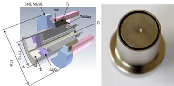
Figure 1: Beam Position Monitor (BPM) for the LHC collimators.
