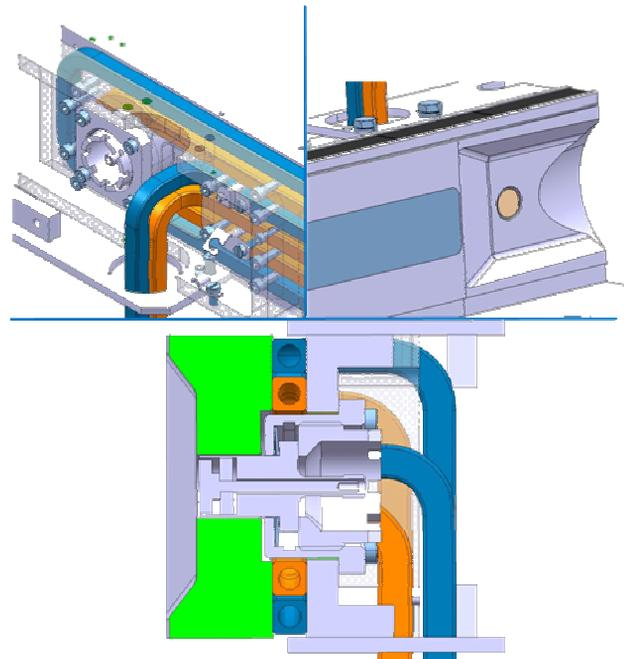
Figure 4: Jaw tapering of future LHC tertiary collimators with BPM housing and fine positioning system.
