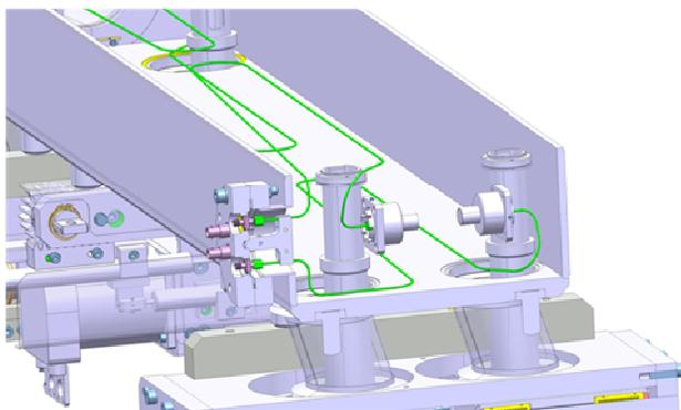
Figure 6: Vacuum tank with layout of coaxial cables and pickup assembly.
