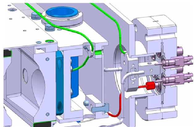
Figure 5: Cross-section of special flange with BPM cable feedthroughs.
