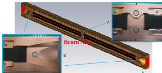
Figure 2: Jaw mock-up embedding four BPMs.
