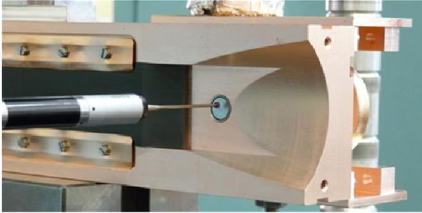
Figure 3: Metrology control of jaw mock-up to check the alignment of the BPM button surface with respect to the surrounding tapering.
