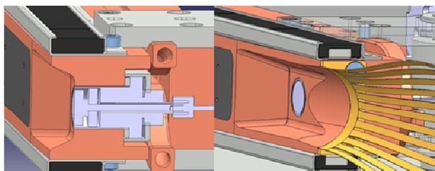
Figure 8: Special collimator for dispersion suppressor
