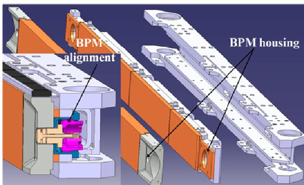
Figure 7: Phase II collimator jaws: tapering with housing and fine positioning system for BPMs.
