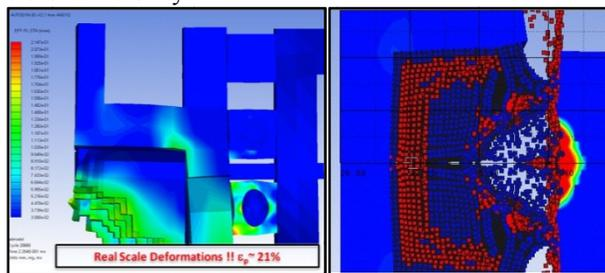
Figures 5 and 6: Case 7. Plastic strain in Cu and Cu-Ni (left) and damage extension on the two jaws (right).
