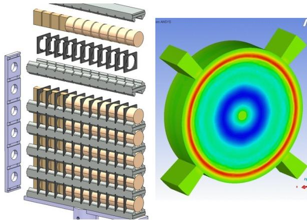
Figures 7 and 8: HiRadMat test bench showing material samples and graphite holders (left). Propagation of a shock wave in a cylindrical material sample (right): note how the graphite holders, thanks to their low shock impedance, do not affect the shock wave pattern.
