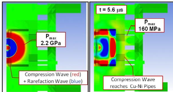
Figures 1 and 2: Case 4. Propagation of the shock wave in the jaw assembly. Note the wave is mostly reflected at the W-Cu interface, only partially transmitted to Cu support.
