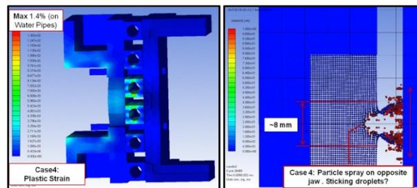
Figures 3 and 4: Case 4. Residual Plastic strain on Cu and damage extension on W. Note how the SPH model allows particles sprayed on the opposite jaw to be visualized.
