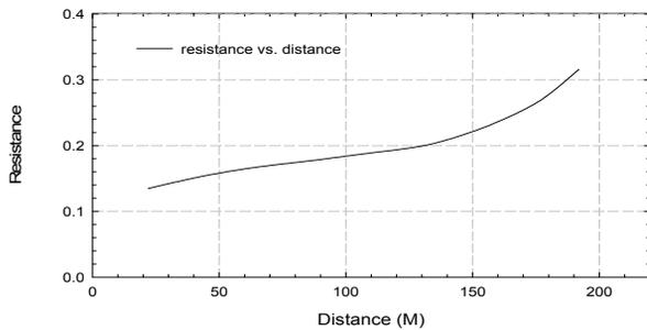
Figure 3: A ground resistance curve measured at region 2 of TPS construction site.
