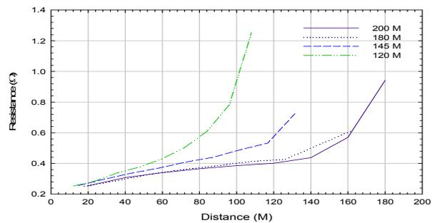
Figure 4: Four ground resistance curves for different distances of E electrode to C electrode measured at the region 5 of TPS construction site.
