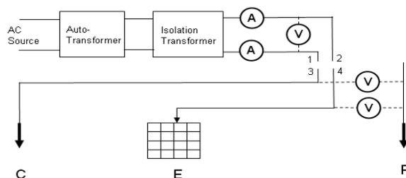
Figure 6: Block diagram for setting up the instruments used in the test-current-reversal method.
