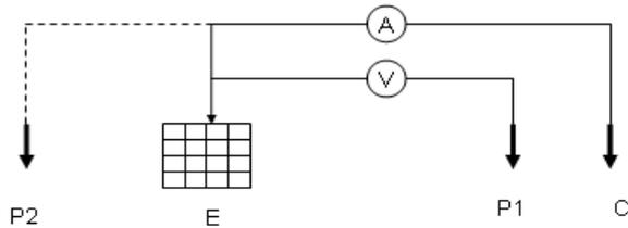
Figure 2: Layout of electrodes and meters for the fall-of-potential method, where E is for the ground grid, C is for the current electrode, P is for the potential electrode, A and V are for the current and the voltage measured by the ground test meter.
