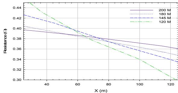
Figure 5: Intersection curves for Fig. 4. The center of the triangle formed by the intersection gives the ground resistance 0.38 Ω.
