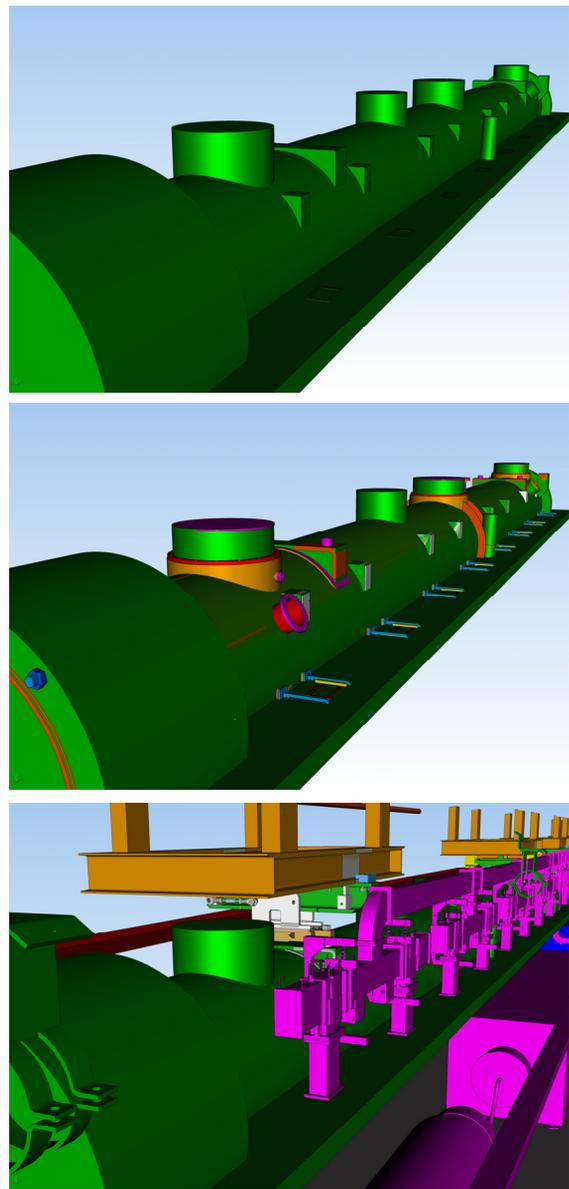
Figure 2: Accelerator module placeholder (top) with rf interface details (middle) and connected waveguides (bottom).
