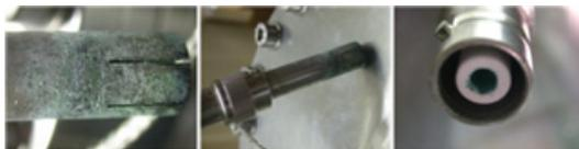
Figure 5: degradation of the outer coaxial surface
