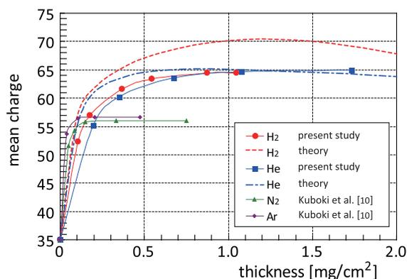
Figure 3: Measured and calculated charge state evolution.
