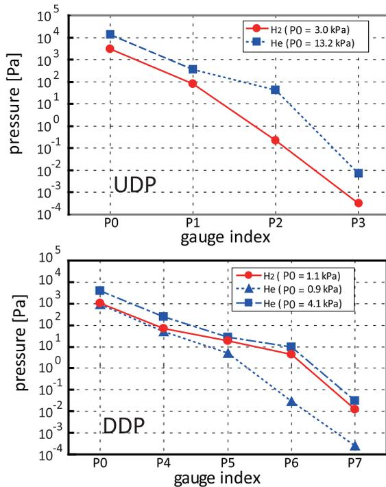
Figure 2: Pressure distributions in the UDP and DDP.
