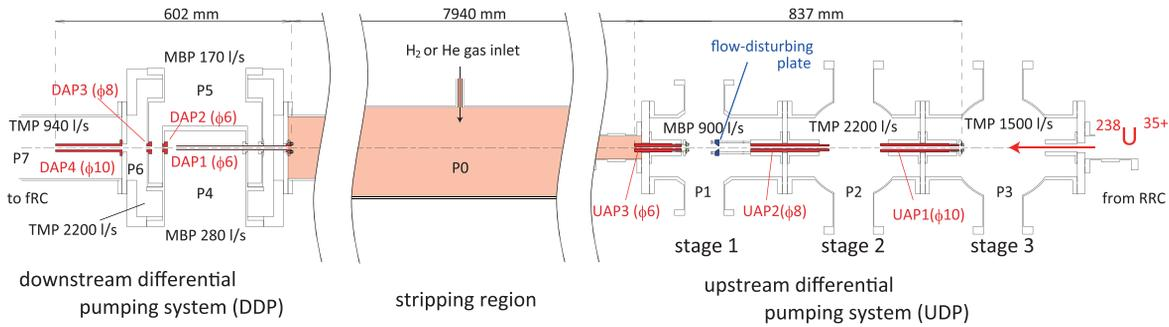
Figure 1: Cross-sectional view of the charge stripping system.
