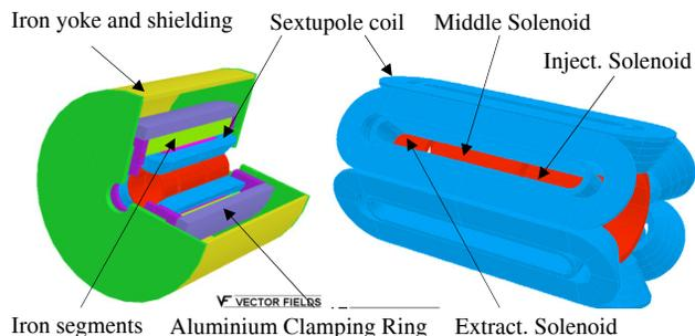
Figure 2: SECRAL superconducting magnet structure.
