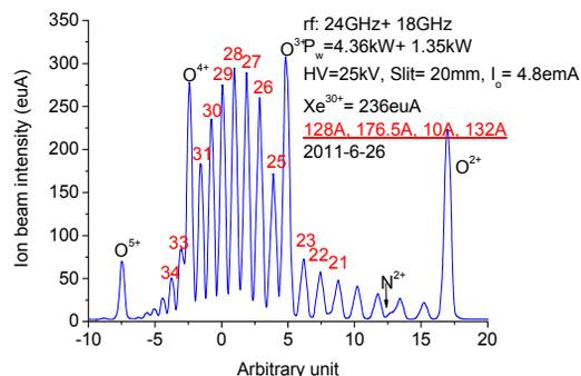
Figure 6: Xe spectrum of SECRAL optimized for  $^{129}\text{Xe}^{30+}$  with double-frequency (24+18 GHz) heating with an aluminium plasma chamber.
