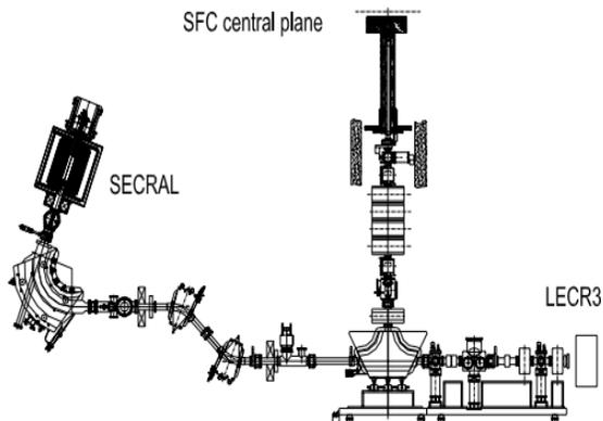
Figure 3: Layout of the axial injection beam line of SFC with two ECR ion sources: SECRAL and LECR3.
