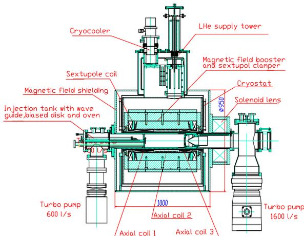
Figure 1: Elevation view of the SECRAL ECR ion source.
