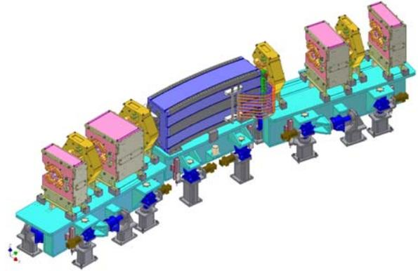
Figure 1: Girder layout for half cell of the storage ring.
