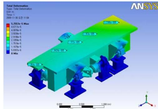
Figure 4: Displacement of MMG.
