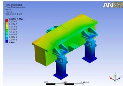
Figure 5: Displacement of MMG.
