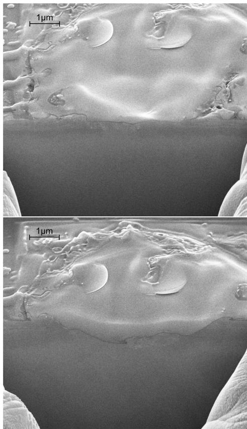
Figure 6: Two pictures of a sequence from a cut and slice analysis of a breakdown site using the FIB at Uppsala University.
