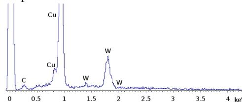
Figure 5: EDX spectrum acquired from the point 2 in Fig. 3. Cu and W peaks are visible.
