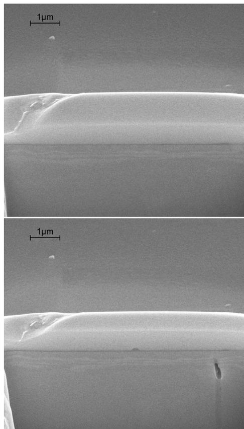
Figure 7: Two pictures of a cut and slice analysis of a pristine location of the diamond turned copper sample.
