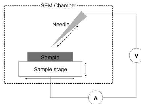
Figure 1: Schematic of experimental setup for field emission measurements and breakdown study.
