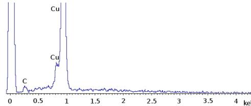
Figure 4: EDX spectra acquired from the point 1 in Fig. 3. Only Cu peaks are visible.
