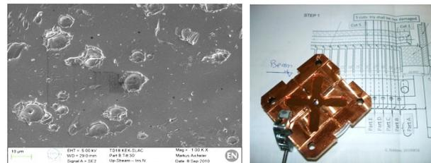
Figure 4: Observation of tested and opened structures, SEM of breakdowns feature.
