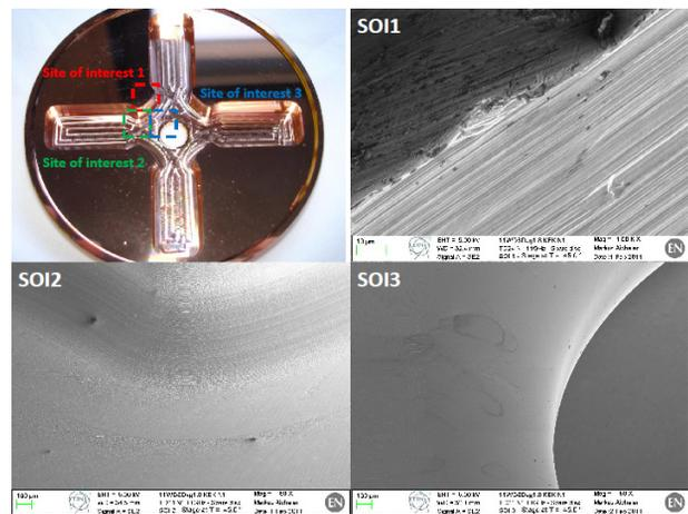
Figure 3: Standard designation of SOI. SOI1: burrs inspection on the top plan; SOI2: radii milling transitions; and SOI3: turning milling transition in the iris.
