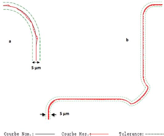
Figure 5: Dimensional plot showing the achieved shape (red) regarding the nominal path (black) and specified tolerances (green): a) iris; b) waveguide.
