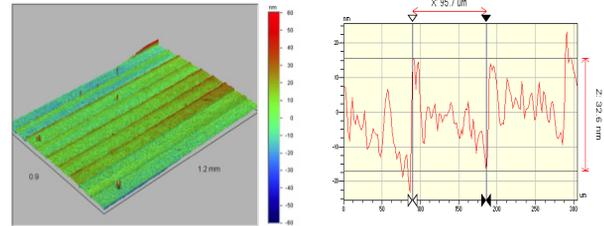
Figure 7: Roughness profile in the milled zone of the waveguide of a damped-disc.  $Ra 5 \text{ nm}$  and  $Rt 36 \text{ nm}$  are measured.
