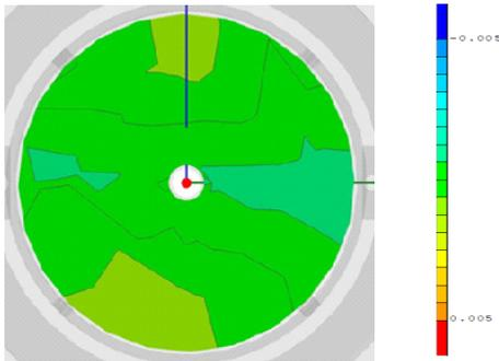
Figure 6: Surface flatness profile of reference face A, scale in mm.
