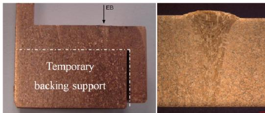
Figure 4: Cross-section of the weld before (left) and after (right) removing the backing support.
