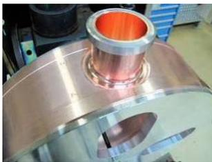
Figure 3: EB welding of ports from the outside.
