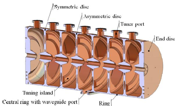
Figure 1: 3D-view of the full prototype PIMS cavity.
