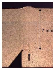
Figure 7: Cross-section of a junction ring to disc EB weld.
