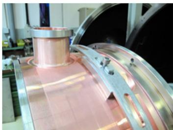
Figure 8: Alignment tooling in contact with the reference diameters of the disc and ring.
