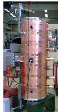
Figure 6: The first tuning step: bead-pull measurements on the clamped PIMS prototype before welding.
