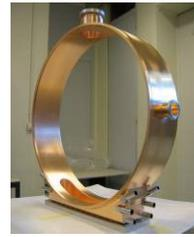
Figure 5: Vacuum brazing of ports on the central ring.
