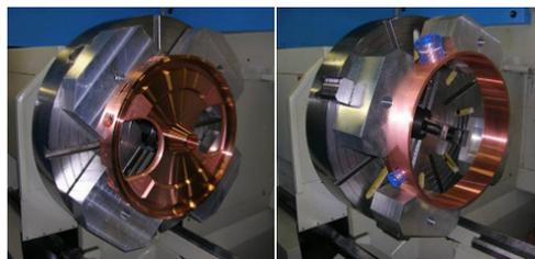
Figure 2: Machining of the discs and rings using aluminium clamping jaws.
