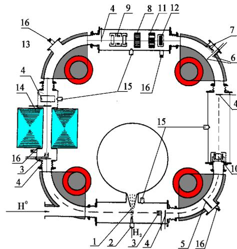
Figure 1: Schematic of storage ring with diagnostics and control. 1-striping gas target; 2-gas pulser; 3-Faraday Cup; 4-Quartz screen; 5, 6-moving targets; 7-ion collectors; 8-current monitor; 9-Beam Position Monitor; 10-Quadrupol pick ups; 11-magnetic BPM; 12-beam loss monitor; 13-detector of secondary particles density; 14-inductor core; 15-gas pulses; 16-gas leaks.
