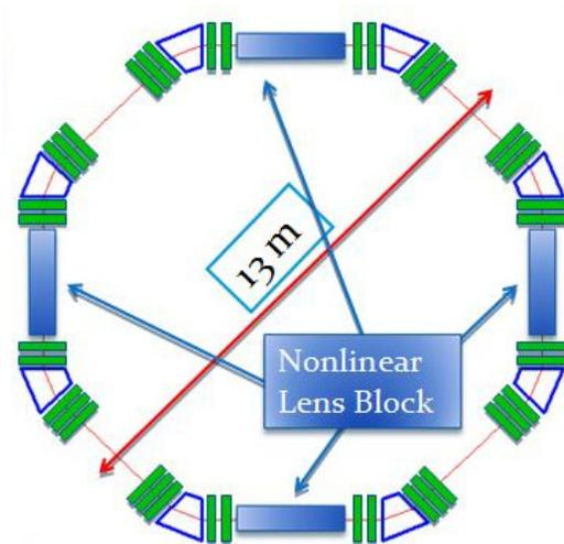
Figure 2: Schematic of storage ring with a nonlinear close to integrable focusing system from [16].
