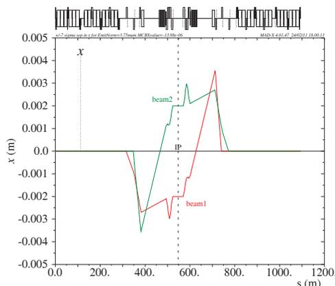
Figure 3: Horizontal separation bump at IP1. The separation is  $\pm 2$  mm at the IP which corresponds to  $\pm 6.65\sigma$  at 3.5 TeV at  $\beta^* = 90$  m for a normalized emittance of  $\epsilon_N = 3.75 \mu\text{m}$ .
