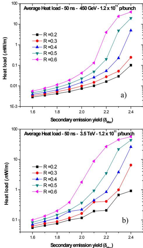
Figure 3: Simulated average arc heat load for 50 ns bunch spacing at a) injection energy and b) top energy.
