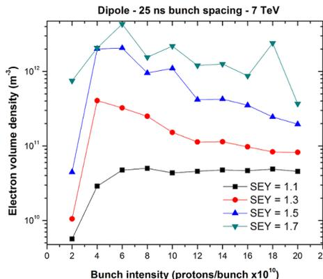
Figure 6: Average electron volume density for a dipole at 25 ns bunch spacing and 7 TeV.
