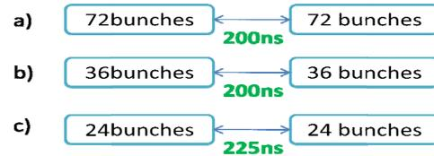
Figure 2: Filling patterns used in simulations for a bunch spacing of a) 25 ns, b) 50 ns and c) 75 ns.
