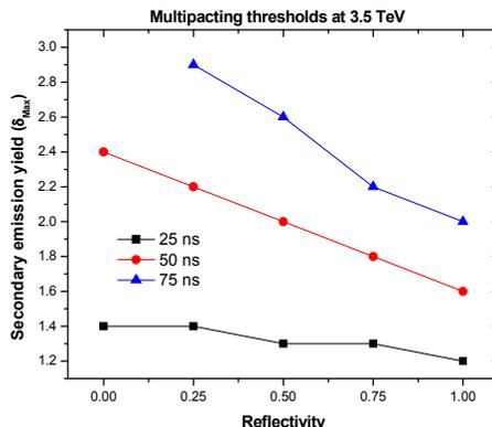
Figure 5: Simulated multipacting thresholds as a function of the electron reflectivity at 3.5 TeV beam energy for three different values of bunch spacing.
