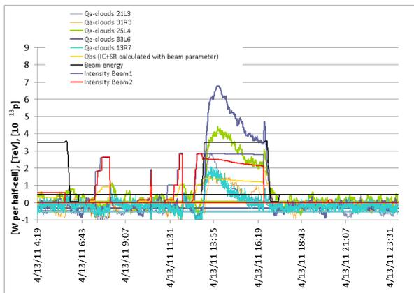
Figure 1: Measured heat load due to the electron cloud during the scrubbing process at 50 ns on April 13<sup>th</sup>, 2011.
