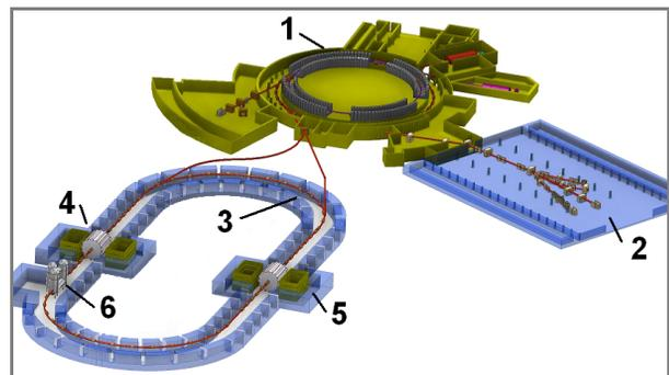
Figure 1: The NICA facility: 1 - the existing accelerator building; 2 - fixed target experimental hall; 3 – collider ring; 4 and 5 - the MPD and SPD detector facilities respectively; 6 – high voltage electron cooling system.
