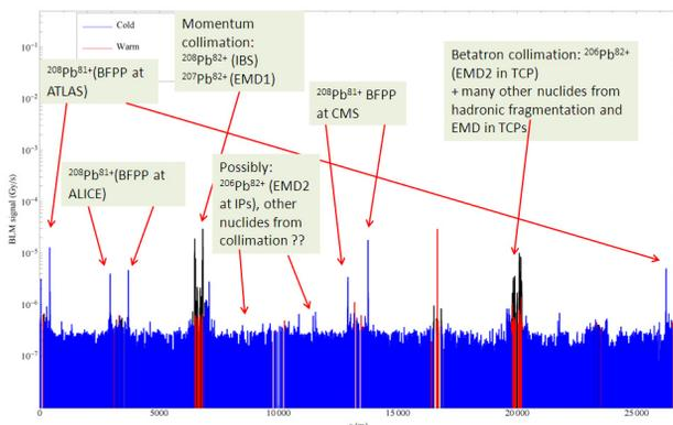
Figure 5: Global view of losses with Pb-Pb stable beams, in the Fill 1541, the last of 2010, which provided record luminosity. The identification of the loss peaks is done according to long-standing expectations.
