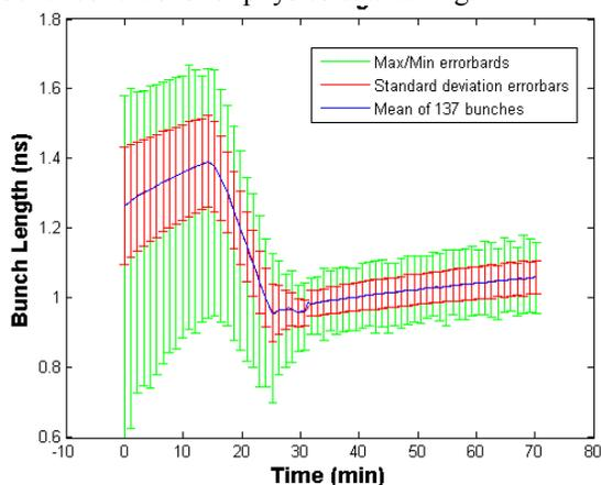
Figure 4: Statistics on bunch length (mean, min, max and standard deviation as error bars) during the ramp (Beam 1, Fill 1539,  $k_b = 137$ ).
