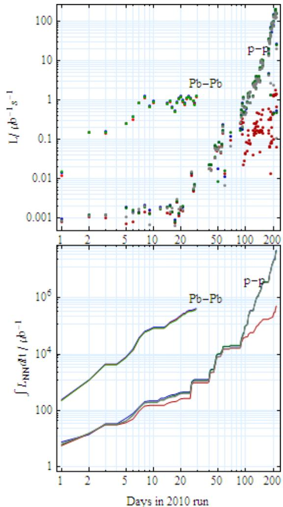
Figure 1: Peak (per fill) and integrated *nucleon-nucleon* luminosity for Pb-Pb collisions (upper, indistinguishable data sets) and p-p collisions during the 2010 runs in ATLAS (blue), ALICE (red) and CMS (green). Days are counted from the first declaration of “Stable Beams”.
