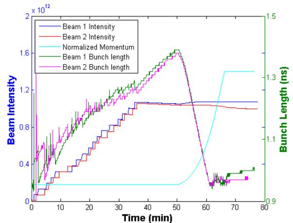
Figure 3: Capture with  $V_{\text{RF}} = 7 \text{ MV}$ , increased to 12 MV through the ramp with longitudinal blow-up on; Fill 1539,  $k_b = 137$  (intensity given in units of charge, not reliable in ramp because of bunch-length change).
