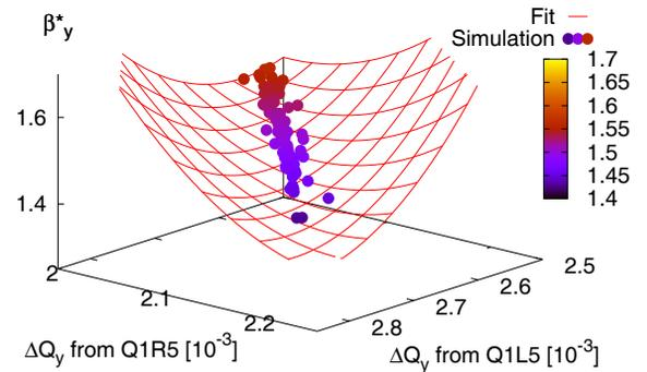
Figure 1: IP5 vertical  $\beta^*$  versus tune-shifts from a change of  $\Delta K = 10^{-5} \text{ m}^{-2}$  in the left and right Q1 quadrupoles. The nominal lattice has  $\beta^*=1.5$  m and random errors around the ring are considered.
