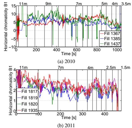
Figure 5: Continuous measurements of chromaticity, similar behavior is observed for the other beam and other plane.
