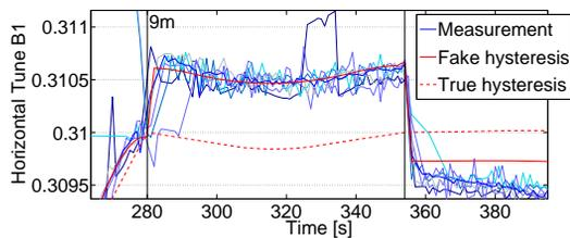
Figure 7: Simulation of tune using MADX, introducing fake changes of hysteresis branch in the settings compared with measurements.
