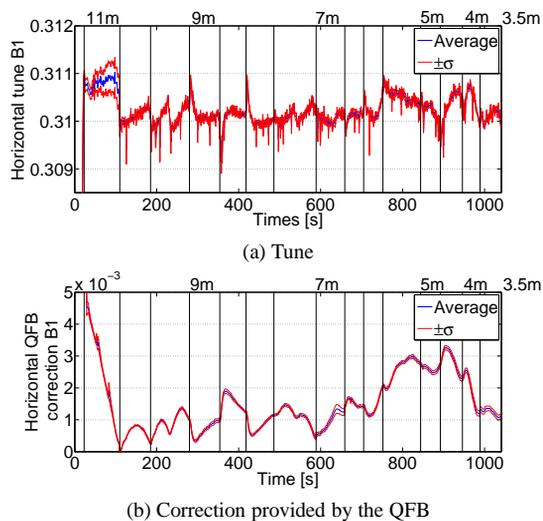
Figure 3: Average over the last 15 fills for physics with proton in 2010 of horizontal tune and correction from the QFB of beam 1. Similar behavior is observed for the other beam and other plane.
