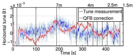
Figure 4: Average over 25 fills for physics in August 2011 of the measured difference to the nominal tune and corrections provided by the QFB.
