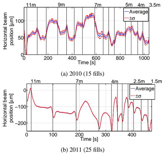
Figure 2: Average over fills for physics with proton of the measured beam position 18m downstream the primary collimators of beam 1.
