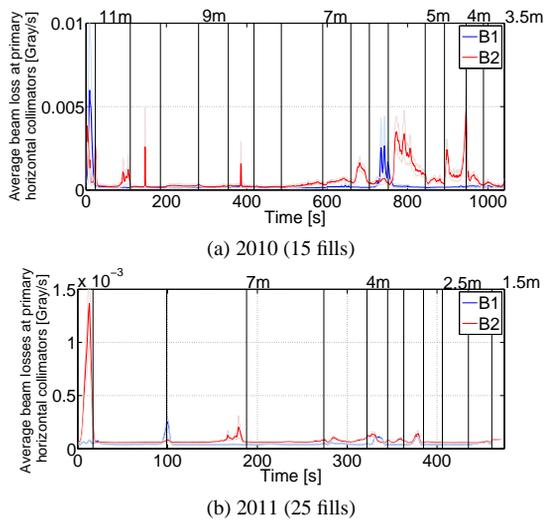
Figure 6: Average over fills for production of physics of the losses detected at the primary horizontal collimator, normalized with the beam intensity at the beginning of the squeeze and scaled to the nominal intensity.
