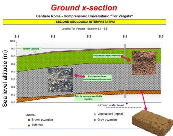
Figure 2: Ground cross section at the Tor Vergata site.
