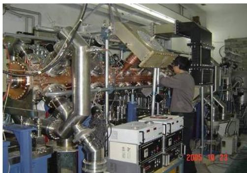
Figure 6: A proton RFQ of 3.5MeV for ADS study has been built at IHEP with 46mA output beam at a transmission rate >93%.
