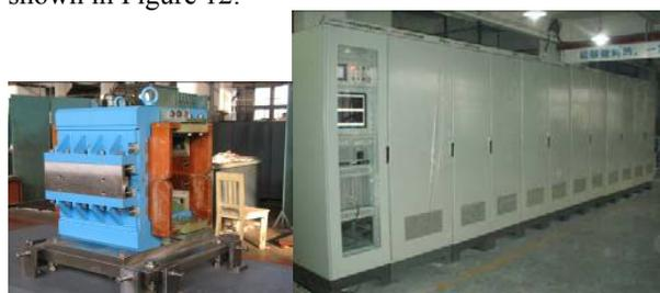
Figure 12: Prototype of the injection bumper and its power supply.
