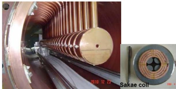
Figure 7: DTL prototype with Sakae coil
