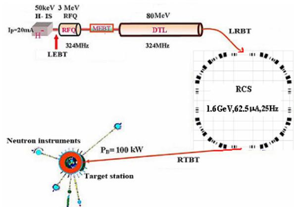
Figure 1: Schematics of the CSNS complex.
