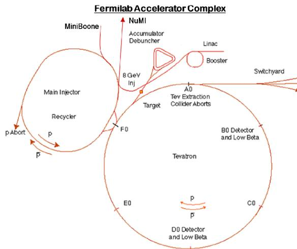
Figure 1: Layout of the Fermilab accelerator complex.
