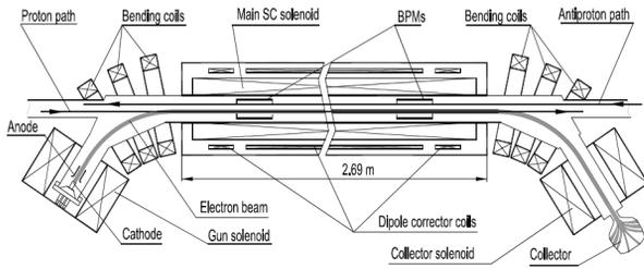
Figure 10: General layout of the Tevatron Electron Lens.
