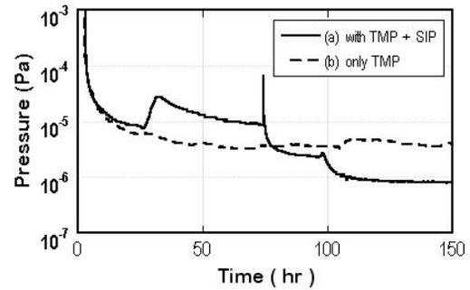
Figure 3: Typical pumping down curves; (a) with ion pumps, and (b) without ion pumps.
