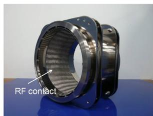
Figure 2: A new type of RF contact which was set in the bellows. This contact is made of Ti braid.
