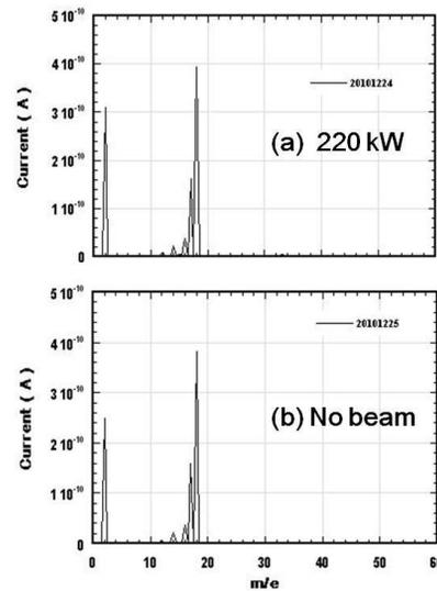
Figure 4: Changes in the residual gas spectra; (a) during the beam operation with the power of 220 kW (24 Dec 2010), and (b) after the beam operation at 220 kW (25 Dec 2010).
