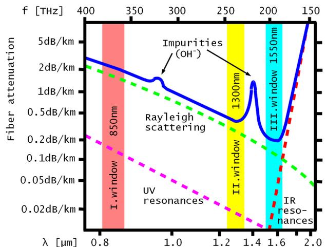
Figure 4: Silica-glass fiber attenuation.
