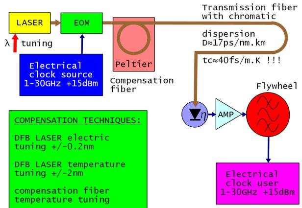
Figure 9: Delay-variation compensation techniques.
