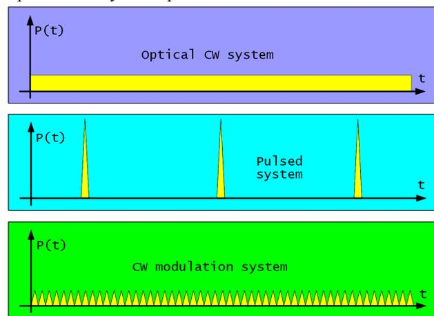
Figure 6: Optical timing systems.
