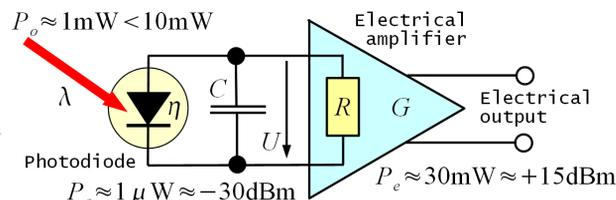
Figure 7: Photo-diode receiver.
