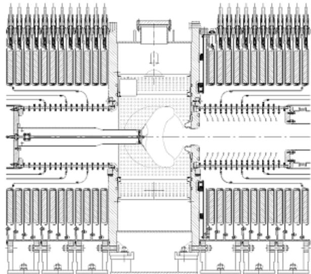
Figure 1: Scheme of LIA-2 accelerating system.
