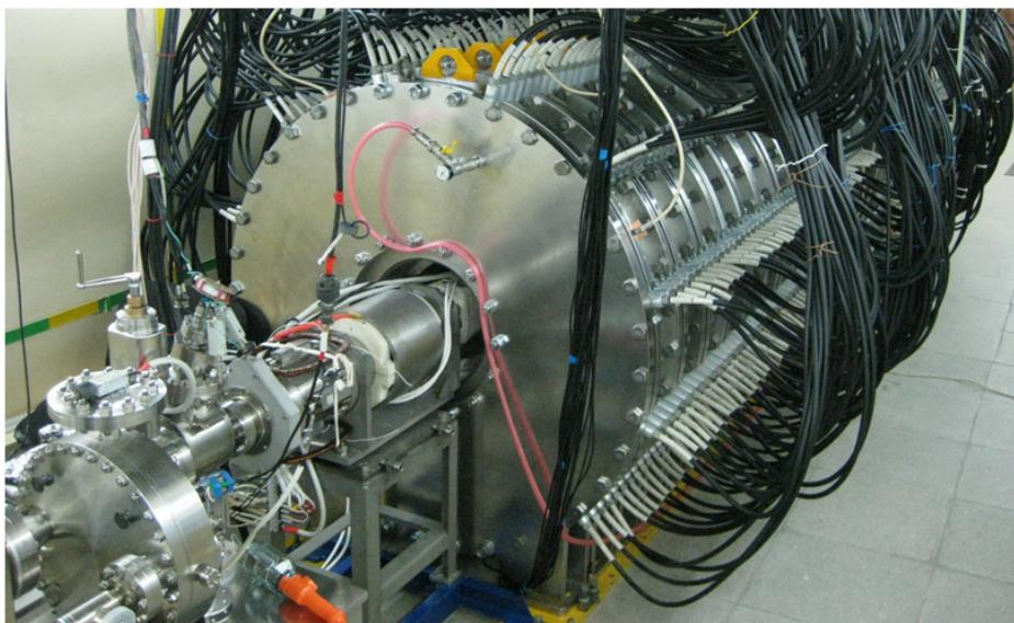
Figure 3: LIA-2 accelerating system and target assembly.
