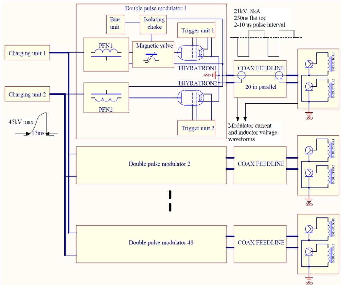
Figure 2: Scheme of LIA-2 pulsed high voltage system.
