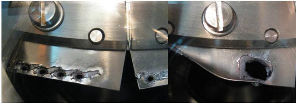
Figure 5: The results of beam interaction with 0.5 mm thick tantalum target for best beam focusing (on the left, 6 shots) and for smaller than optimum current in final focusing lens (on the right, 1 shot). All other parameters are the same for all shots and correspond to maximum beam energy and current (see Fig. 3). Bolt head diameter on the picture is equal to 8.5 mm, pin diameter – 4 mm.
