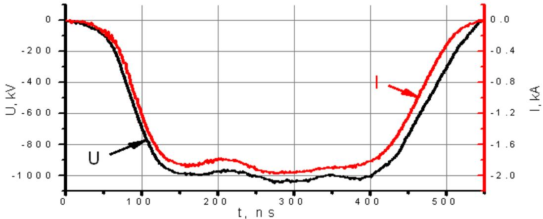
Figure 4: Oscillograms of voltage (black) and current (red) of LIA-2 diode.
