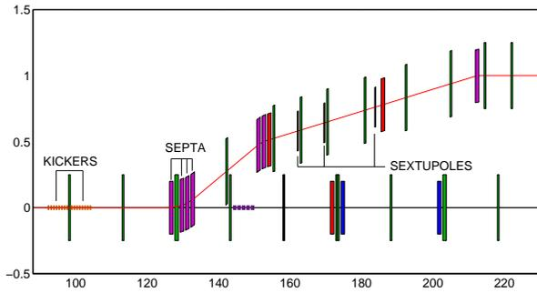
Figure 4: Side view of the separation area between the straight line and the dump line TLD. Green and red/magenta colors mark quadrupoles and horizontal/vertical dipoles.
