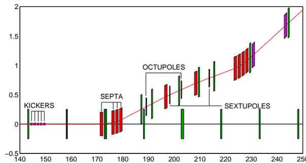
Figure 2: Top view of the separation area between the straight line and the beamline TD1. Green and red/magenta colors mark quadrupoles and horizontal/vertical dipoles. Horizontal and vertical distances are measured in meters.
