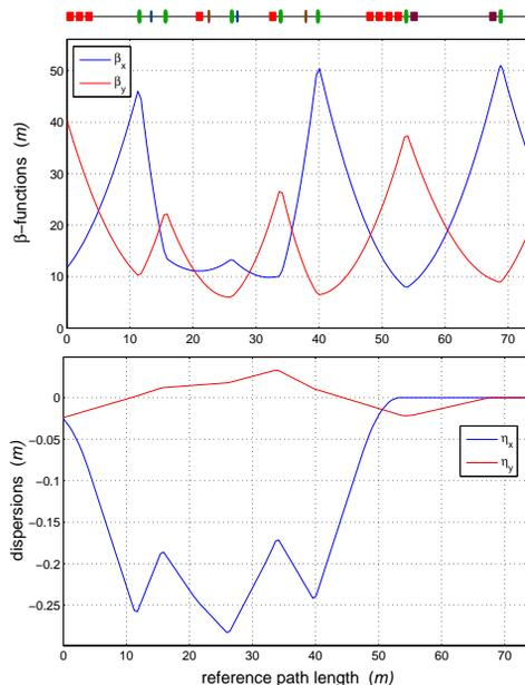
Figure 3: Betatron and dispersion functions along the deflection arc TD1 shown starting from the entrance of the first untilted septum.
