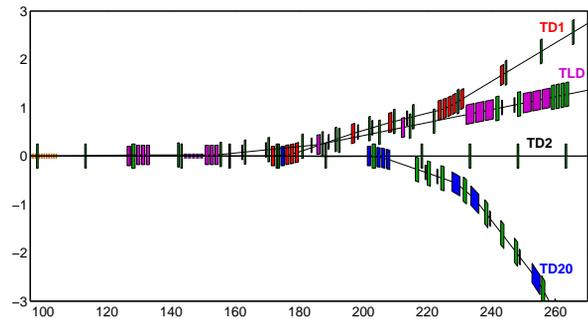
Figure 7: Top view of the separation area. Red, magenta and blue colors mark septa and dipoles of beamlines TD1, TLD and TD20, respectively. Horizontal and vertical distances are measured in meters.
