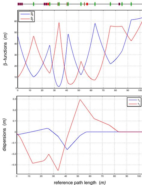
Figure 5: Betatron and dispersion functions along the deflection arc into the dump line TLD shown starting from the entrance of the first untilted septum.
