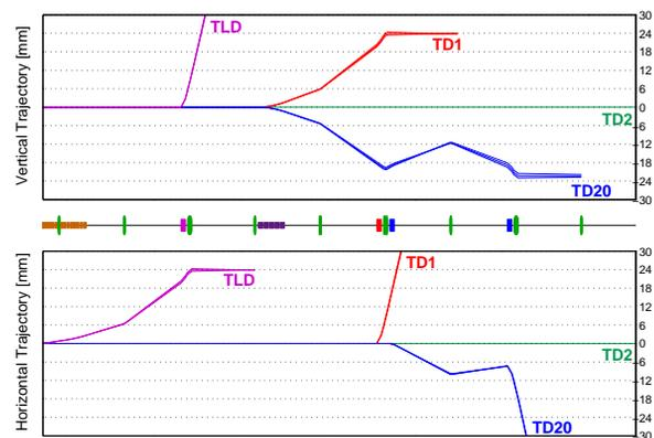
Figure 1: Trajectories of kicked particles (with the relative energy deviations of  $-1.5\%$ ,  $0\%$  and  $+1.5\%$ ) in the separation area. Magenta, red and blue colors mark the extractions into the dump line TLD, the undulator beamline TD1, and the future line TD20, respectively. Green color marks the straight line TD2.
