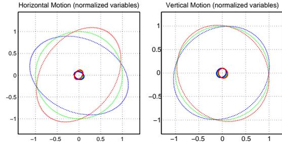
Figure 6: Phase space portraits of monochromatic  $0.1\sigma_{x,y}$  and  $1\sigma_{x,y}$  ellipses (matched at the entrance) after tracking through the extraction arc into the dump line TLD. The relative energy deviations are equal to  $-1.5\%$ ,  $0\%$  and  $+1.5\%$  (red, green and blue ellipses, respectively).
