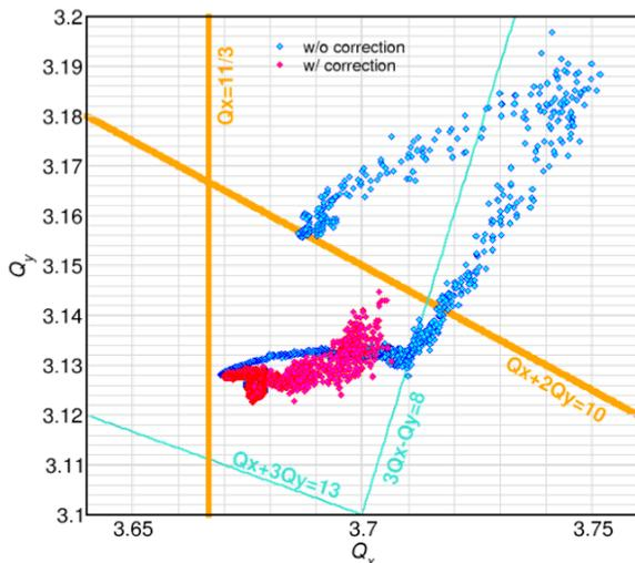
Fig. 6: Tune diagram for the tracking results.
