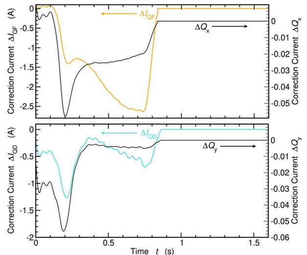
Fig. 4: Correction current for QF and QD magnet.
