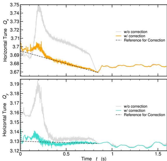
Fig. 5: Correction results of the time profile of the horizontal/vertical tune.
