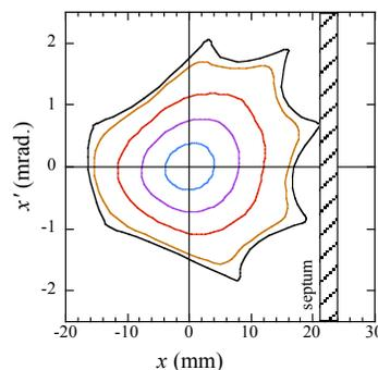
Figure 3: Phase space contour at the injection point of NewSUBARU. The shaded area is the injection septum.
