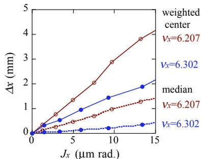
Figure 5:  $J_x$  dependence of the weighted center and the median of the stored beam at NewSUBARU for  $v_x = 6.302$  and  $v_x = 6.207$ .
