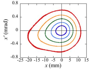
Figure 6: Phase space contour at the injection point of SPring-8 SR.
