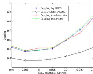
Figure 10: The coupling changed by different skew quadrupole strength.
