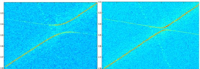
Figure 5: The betatron coupling correction result.
