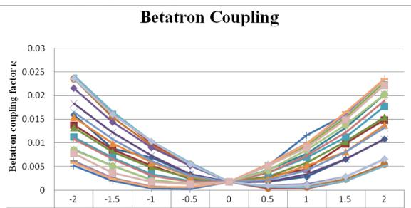
Figure 3: The betatron coupling responds to the skew quadrupole current.
