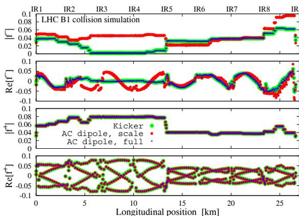
Figure 4: CRDTs in a simulated lattice reconstructed from the kick and AC dipole excitations. Skew quadrupole errors are based on the measurement in Fig 3.
