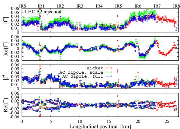
Figure 2: Another example of CRDTs measured with the kickers and AC dipoles. The full calculation gives a result closer to that from the kickers in this case.
