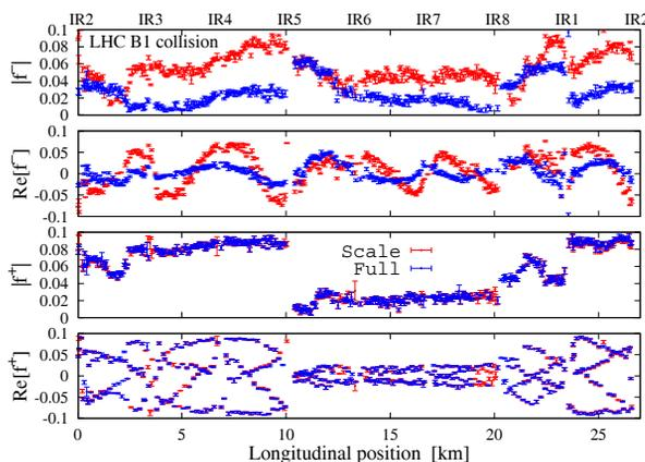
Figure 3: CRDTs of the collision optics of the LHC Beam1. A case where the largest discrepancy between the simple scaling and the full calculation is observed.
