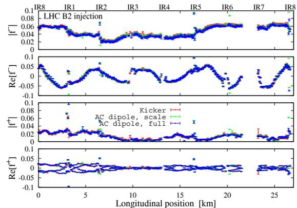
Figure 1: CRDTs of the LHC Beam2 measured with the kickers and AC dipoles. The simple scaling and full calculation provide almost identical result in this case.
