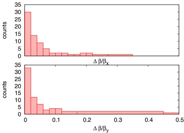
Figure 5: Histogram of the difference in the  $\beta$ -beat. Top horizontal plane and bottom vertical plane. Horizontal label is the difference in the  $\beta$ -beat between two fills separated by 6 weeks.
