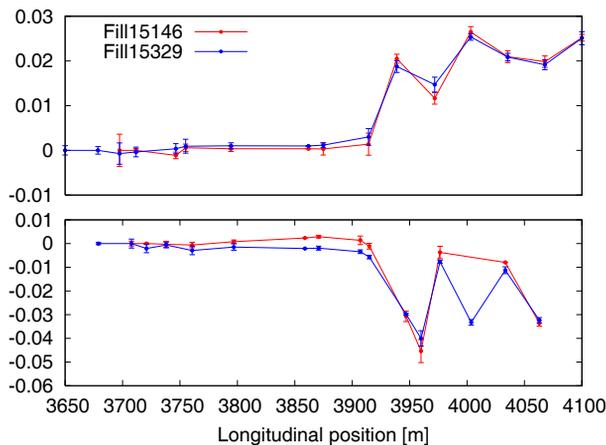
Figure 6: Measurement for the phase error in  $IP_6$  is shown. The horizontal plane, top and vertical plane, bottom. Different starting BPMs were used and measurements were separated by 6 weeks. In the vertical plane there is one missing BPM for fill15329, compared to fill 15220.
