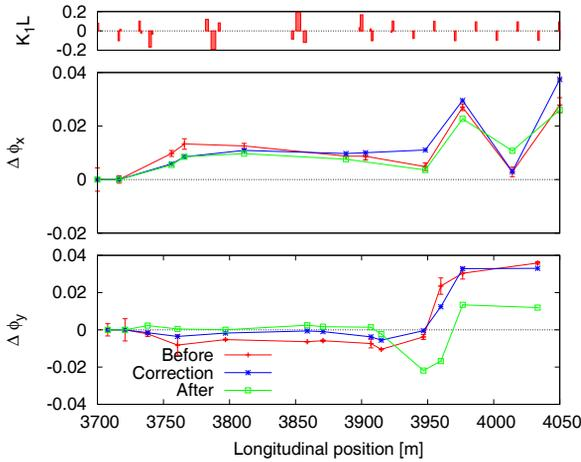
Figure 2: Local correction for  $IP_6$ . Small plot is the location and strengths of the quadrupoles around the ring. Top plot is horizontal plane and bottom vertical plane. Measurement before correction (red), fitted model (blue) and measured after correction (green). Largest deviation is observed in the vertical plane.
