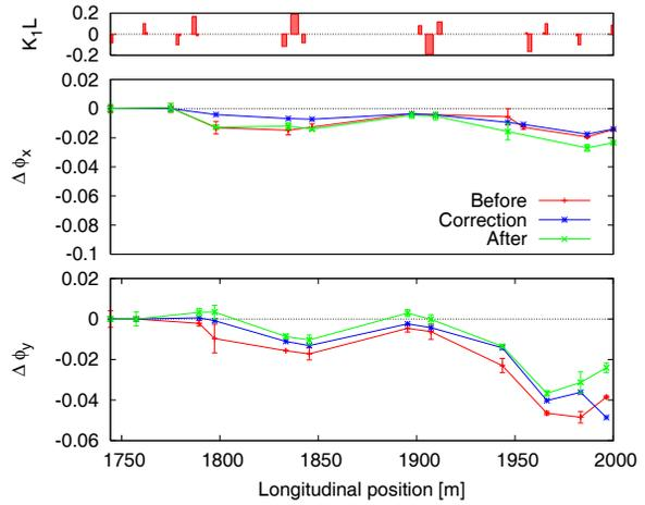
Figure 3: Local correction for  $IP_{12}$ . Small plots are the location and strengths of the quadrupoles around the ring. The large top plot is the horizontal plane and bottom vertical plane. Measurement before correction (red), fitted model (blue) and measurement after correction (green). Largest error is observed in vertical plane.
