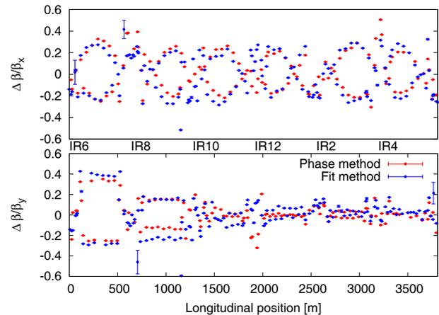
Figure 1: Comparison between the two different methods used to measure the optics at RHIC. Horizontal plane, above and vertical plane, below. Abrupt jumps are observed in the vertical plane for  $IP_6$ ,  $IP_8$  and  $IP_{10}$
