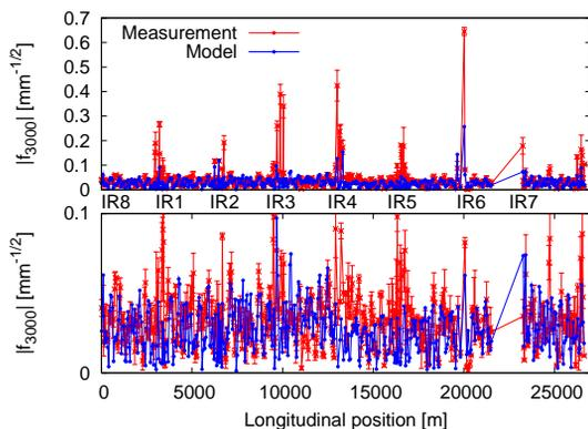
Figure 3: The absolute value of the  $f_{3000}$  resonance driving term is shown. Top plot including large values around the IPs and bottom zoom on the arcs. The gap in the data is due to some missing BPMs. Measurement (red) and model (blue), in the arcs, are in relative good agreement. Decoherence factor of 2 is included in the measurement data.
