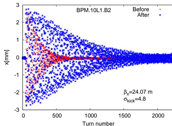
Figure 2: Turn-by-turn data before (red) and after (blue) correction. The decoherence was reduced by a factor of 3.
