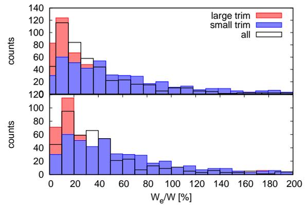
Figure 7: Histogram of the relative error on the chromatic amplitude function for measurement at  $\beta^* = 3.5$  is shown. The error on the measurement is significant. Slightly better result for large trims.
