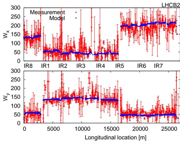
Figure 6: Measurement for the chromatic amplitude function at  $\beta^* = 1.0$  m. Measurement, red and model, blue. Measurement and model are in relative good agreement.
