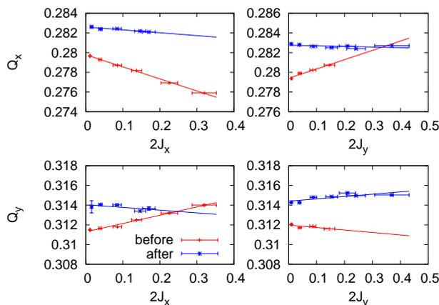
Figure 1: Amplitude detuning before any corrections (red) and after (blue). Horizontal plane (top) and vertical plane (bottom) are shown. A significant reduction is achieved.
