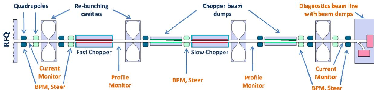
Figure 1: The Medium Energy Beam Transport Line (MEBT)
