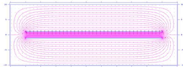
Figure 3: Superfish beam chopper model.
