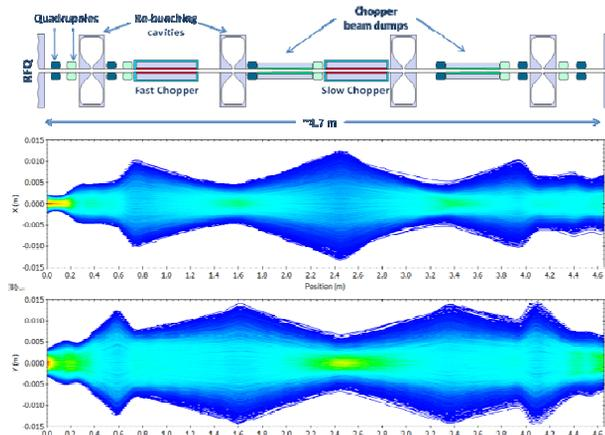
Figure 5: Characteristic particle trajectories through the MEBT line, with the beam choppers switched off (horizontal and vertical planes).
