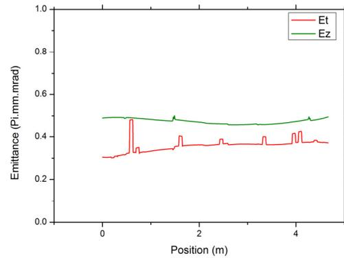
Figure 8: Emittance evolution in the MEBT.
