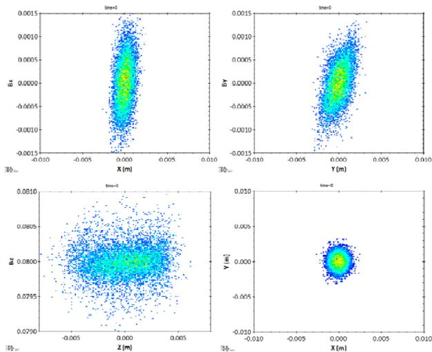
Figure 4: Input MEBT beam distribution:  $\epsilon_t \sim 0.31$  Pi.mm.mrad,  $\epsilon_z \sim 0.18$  Pi.deg.MeV (RMS, Normalised).
