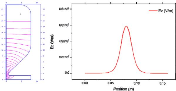
Figure 2: Cavity cross-section as modelled by Superfish and the resulting electric field map on axis.
