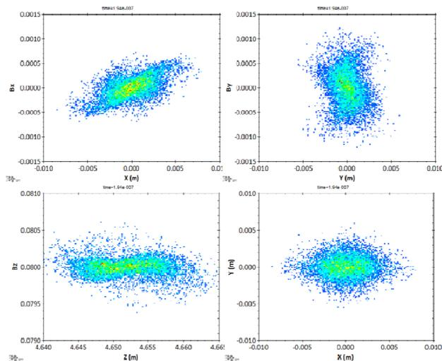
Figure 6: Output MEBT beam distribution:  $\epsilon_t \sim 0.37$  Pi.mm.mrad,  $\epsilon_z \sim 0.18$  Pi.deg.MeV (RMS, Normalised).
