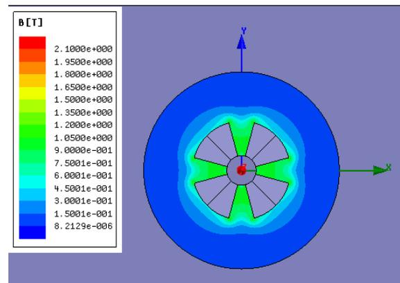
Figure 9: Magnetic field map of the EMQ at 5 A/mm<sup>2</sup>.
