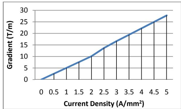
Figure 8: Magnetic field gradient with Current Density (Winding radius = 50 mm, Yoke Outer radius = 100 mm, Angle = 75°).
