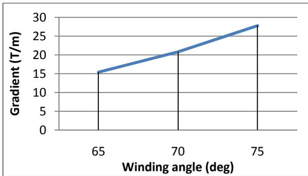
Figure 6: Magnetic field gradient with Winding angle (Current density = 5 A/mm<sup>2</sup>, Yoke Outer radius = 100 mm, Winding radius = 50 mm).
