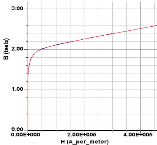
Figure 3: B-H curve for silicon steel M400.
