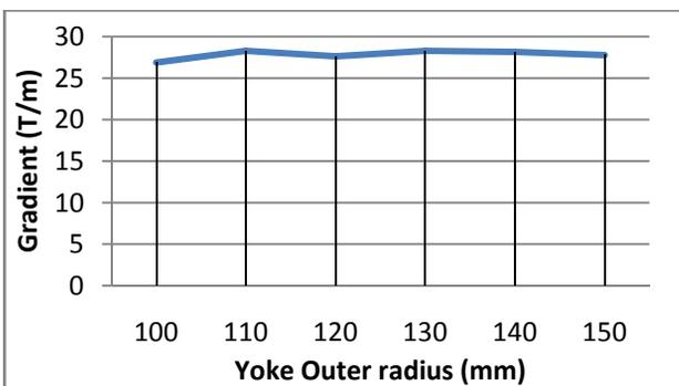
Figure 7: Magnetic field gradient with Yoke Outer radius (Current density = 5 A/mm<sup>2</sup>, Winding radius = 50 mm, Angle = 75°).
