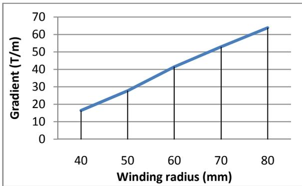
Figure 5: Magnetic field gradient with Winding radius (Current density = 5 A/mm<sup>2</sup>, Yoke Outer radius = 100 mm, Angle = 75°).
