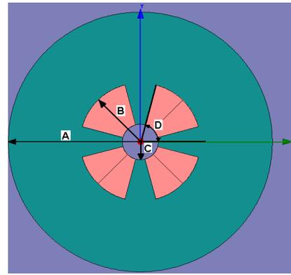
Figure 4: Quadrupole configuration: A) Yoke Outer radius; B) Winding radius; C) Aperture radius; D) Winding angle.
