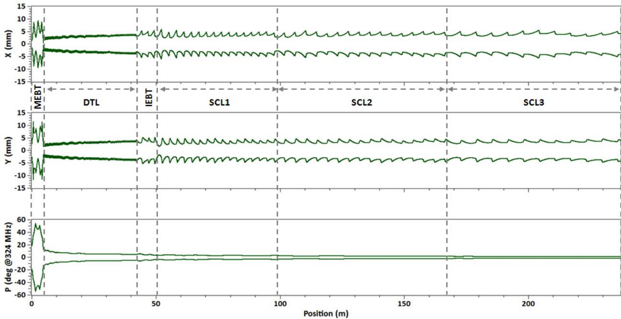
Figure 2: Beam envelopes along the linac (MEBT to SCL3).
