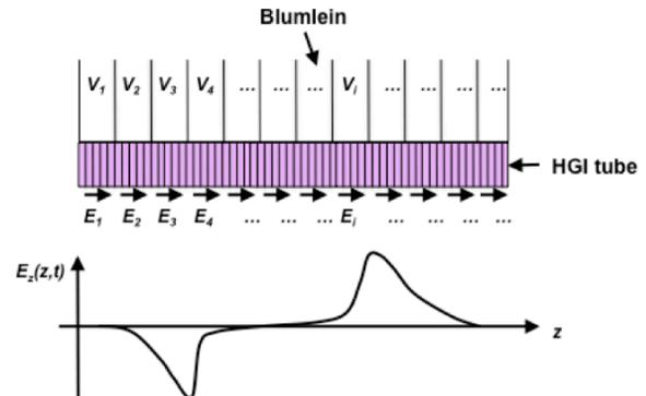
Figure 1: The schematic of a high-gradient electric HGI lens.
