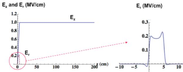
Figure 2: Longitudinal and radial electric field profile.
