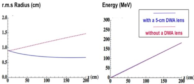
Figure 3: Proton bunch's r.m.s. beam radius and energy in a DWA with a 5-cm electric focusing DWA lens (solid blue) and without a lens.
