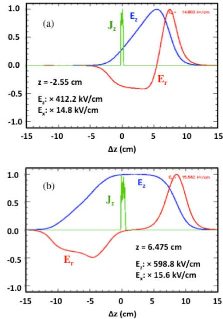
Figure 4: The longitudinal and radial electric field profiles of (a) a strong electric focusing DWA lens at the DWA entrance ( $z = -2.55$  cm) and (b) constant acceleration inside the DWA ( $z = 6.475$  cm) and proton current profiles.
