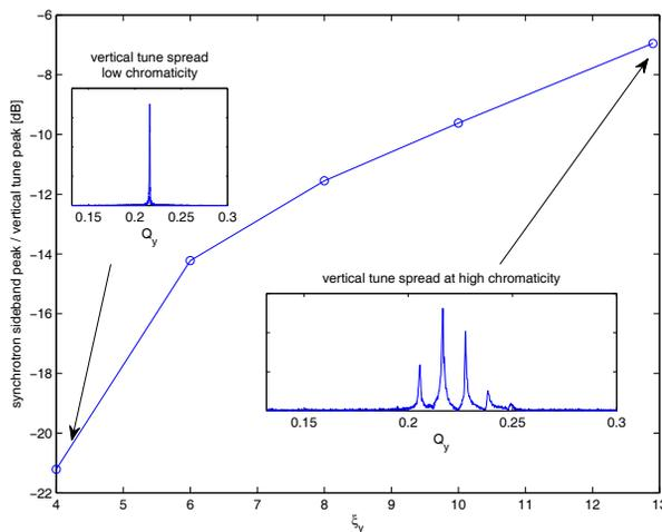
Figure 2: Tune spread vs vertical chromaticity.
