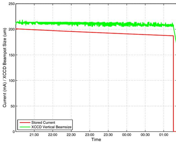
Figure 4: Beam current and vertical beam size during IVU gap scanning.
