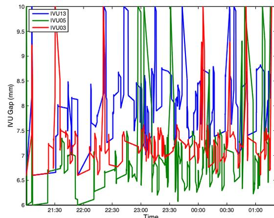
Figure 3: Test of transverse bunch-by-bunch feedback system with varying IVU gaps.
